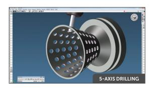
and workholding devices, and automatically corrects the toolpath according to user specified parameters. A sophisticated and powerful programming tool for any 5-axis programmer, this option is ideal for 5-axis simultaneous capable mills, mill-turns and MTM machines, and also a very good solution for 4-axis machines
