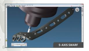
when working directly from solids and surfaces. The integration of 5-Axis Milling with GibbsCAM MTM options supports the most advanced multi-task machines with live tooling on articulated heads. With its breadth of capability and ease of use, GibbsCAM 5-Axis Milling will simplify your 5-axis programming needs and improve machining efficiency with better surface finish and faster throughput.
