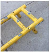
Step 3. Insert two more cross sections into the opposing shoulder section. These two sections will be either male or female internal and allow you to join sections in the middle, lining up the holes in inserting pins.
