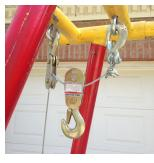
Step 9. Now insert the bottom leg segments making sure that the eyebolts on the bottom are facing inward so that tension chains can be attached. For this step two people are needed, one to hold the unit up, the other to insert the bottom leg segments.
