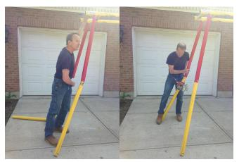
Step 8. Unwind the winch giving you slack on the snatch blocks and end hook. Attach the end hook onto the internal eyebolt on the shoulder, then attached the internal snatch block hook onto the external eyebolt on the shoulder unit. Do this for both winches on each end.
