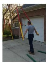
Step 10. The unit is now assembled and is ready to attach the tension chain between the four legs. The tension chain has three pieces. Two separate chain loops with two quick links that attached to the eyebolts on the bottom of the leg.
