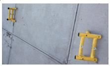
Step 2. Insert two cross brace sections into the inside slots on shoulder sections, lining up pin holes and placing locking pins in both holes. Make sure both cross brace sections are similar, both male or female on the internal ends.
