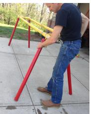
Step 6. The middle leg sections are next. The left side section will have a winch, make sure the winch handle is facing out.
