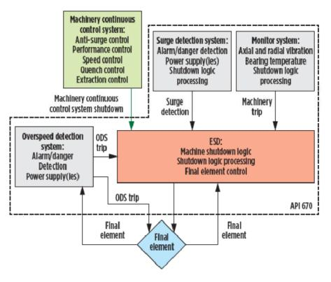
Source: white paper on control and safety for turbo machinery by CCC **Distributed API670 architecture for the MPS**
