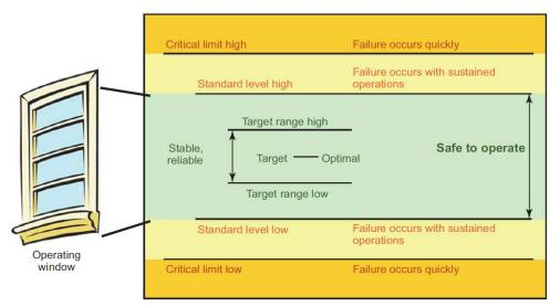
Figure 10 – Integrity operating window definition (Source: API RP 584)
