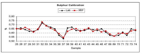
Fig. 9: Online measured sulphur content
