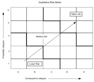
Figure 6 – Example risk matrix using probability and consequence categories to display risk rankings (Source: API RP 580)
