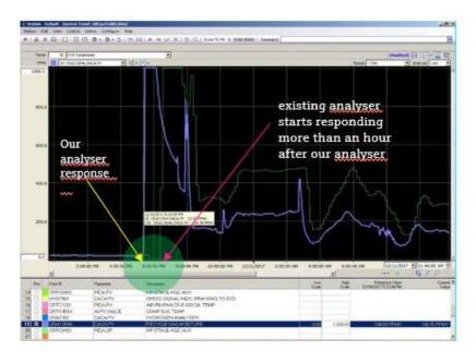
*Fig: 3. TDL analyser picking up a moisture breakthrough event almost an hour earlier than the existing analyser.*
