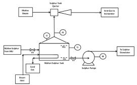
Figure 3. Simplified sketch of the Sulphur tank
