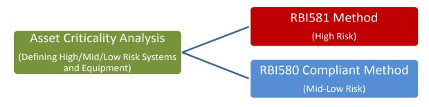
Figure 5 – Proposed workflow of multiple RBI methods being applied concurrently.
