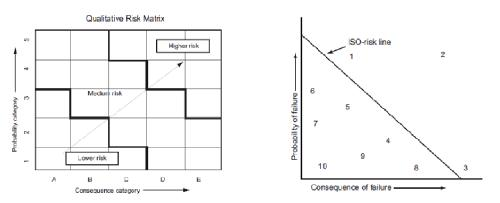
Figure 4 – Outputs of qualitative and quantitative methods respectively. (Source: API RP 580)
