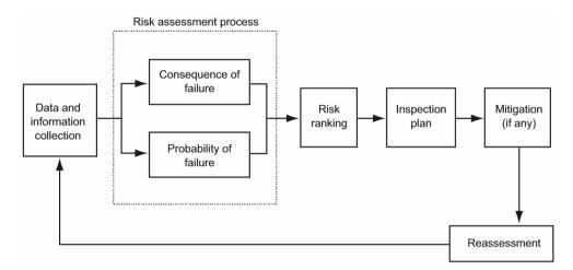
Figure 3 – Risk Based Inspection planning process. (Source: API RP 580)
