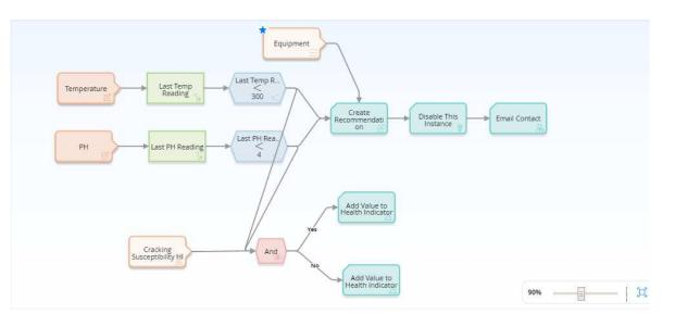
Figure 13 – Policy automating warning based on wet H<sub>2</sub>S potential degradation mechanism.
