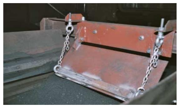
Fig. 4: Hinged plate to smooth the surface
