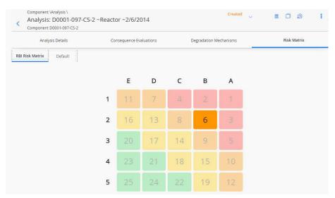
Figure 9 – Expected output from quantitative or semi-qualitative RBI analysis, where the specific risk result is given for the equipment sub-component (e.g. reactor cylindrical shell)
