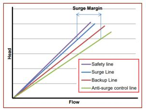
Surgingcan be observed if the flow falls below setpoint andthe Compressor operating point on the curve crossesthe surge line. As the occurrence of surge and itsimpact on the Compressors Gas and the upstreamequipment in various plants is continuingfor a longer period of time, the Compressor control adapts mechanism dvnamic simulation method to facilitate stabilization of the Compressor operation by compensating the disturbances and avoid surge phenomenon.
