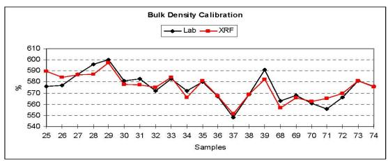
Fig. 8: Online measured bulk density
