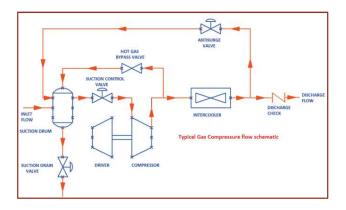
The operating zone of a Compressor is a region constrained on almost all sides by additional boundaries that are to be controlled or at least must be taken in to design. The operation of the Dynamic Compressor can well be represented in the Compressor map, on which the Volumetric flow  $Q_s$  is plotted on X-axis and Compression ratio  $R_{\rm c}$  on Y-axis.
