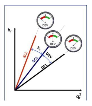
The distance between the Surge Control Line (SCL) and Surge Limit Line (SLL) is mainly a function of the Anti-Surge control system response time, Anti-Surge control valve characteristics, and the control algorithm used.
