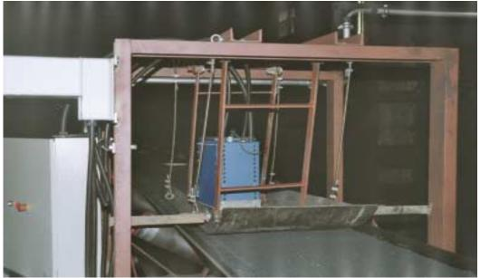
Fig. 3: OXEA® installed on a sled at a main belt of the voestalpine coking plant.
