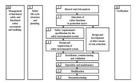
Figure 1. SIS safety life-cycle phases and FSA stages
