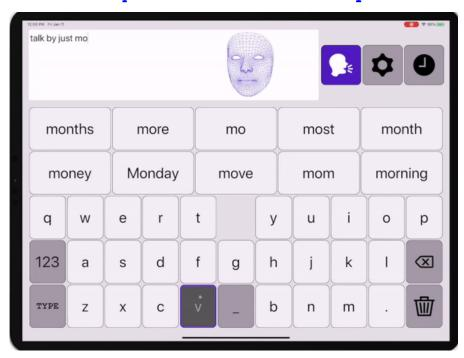
Image shows screen shot of the mobile with alphabets and word prediction and the cursor controlled by head movement
