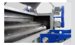
The P pipe shredders are equipped with a special feeding trough sized to take pipes of up to 6 m length. A powerful hydraulic ram forces the pipes into the rotor.
