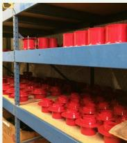
Sight Checks are available in sizes ranging from 2" to 8" diameter. All the components are made in the shop, assembled, painted and stored ready for assembly. As orders come in for the checks, they are assembled by hand and shipped to wholesalers for distribution, not only in Texas, but neighboring states as well, and even into Mexico.
