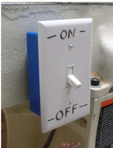
I used a regular el-cheapo light switch in a single blue plastic junction box and screwed a 1" rare earth magnet onto the back of the junction box so that I can place the switch anywhere I want on the lathe. I also used about 6' of regular 2 wire 120 VAC lamp cord (because I had it on hand) to allow me to have the headstock and switch at opposite ends of the lathe at the same time.
