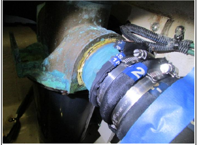
Starboard Main Engine Raw Water Strainer Hose Leak
