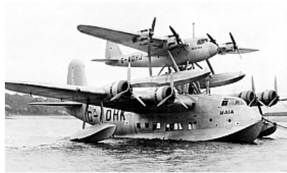
The "Short-Mayo Composite" (designed by Major R.M. Mayo of Imperial Airways). The mother aircraft, Maia, carried the smaller Mercury.
