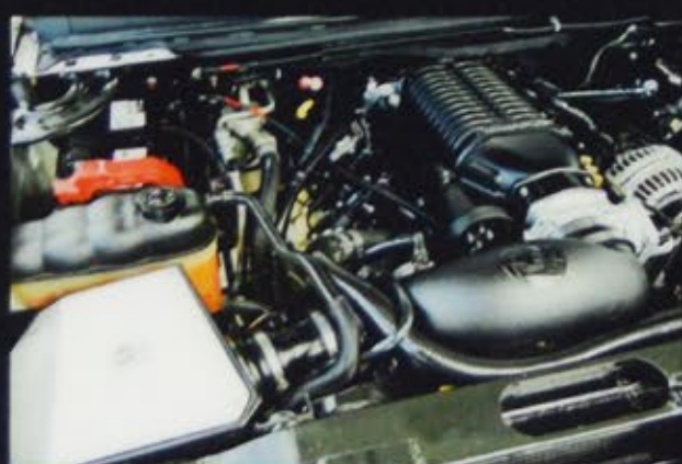
Looks can be deceiving. Hidden under that 2.9L Whipple blower is a fire-breathing 383ci engine capable of unleashing some fury. With 715 hp and 660 lb-ft of torque, that fury comes on in a rage and sounds incredible while doing it.
