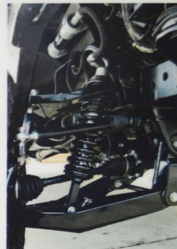
Finding 17 1/2 inches of front wheel travel on a four-wheel drive without modifying the frame is pretty tough. McGaughy's managed to do it with fully fabricated and extended front control arms, custom knuckles riding on beefy Uniballs, and Fox 2.0 coilover shocks with external reservoirs.
