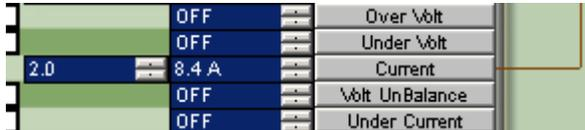
In this example the output is active after 2 seconds when any phase exceeds 8.4Amp.
