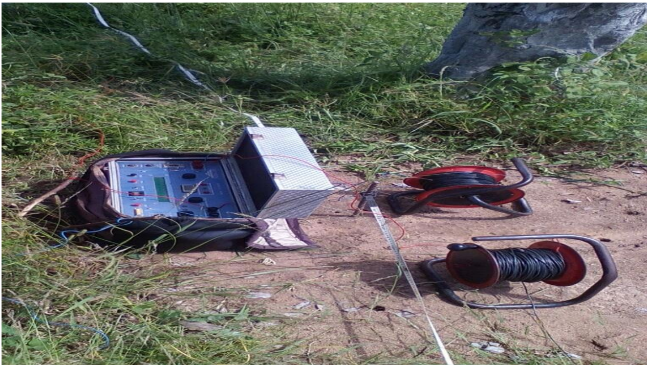
Fig. 1. Connection of the Terrameter in field work
