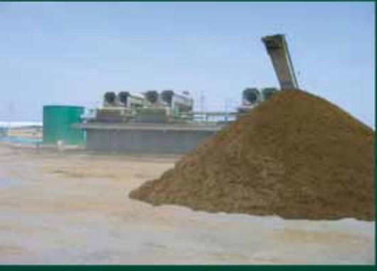
Below: Primary and secondary separators with upflow sand sedimentation tank on Biolyнк system handling the flush manure from 8,000 cows in freestalls in Eastern Oregon.
