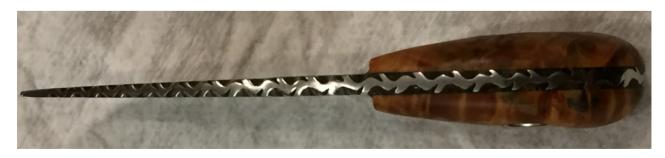
Here is a different version of this using  $\frac{1}{2}$ " spacing on my layout. It is more stretched out and thinner. It also has finger grooves cut in mid-way to add more grip. You can do this just make it blend in with your pattern.
