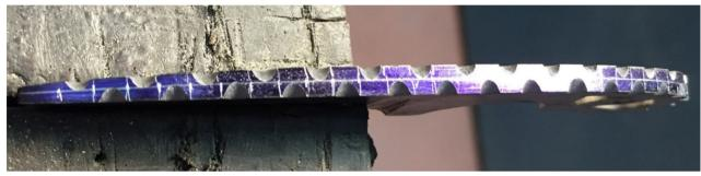
Here you can see how the grid layout helps with the spacing for the half round portions. The half round portion is now done on both sides.
