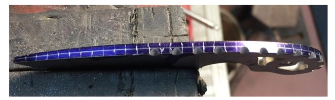
This is a neck knife that shows the  $\frac{1}{4}$ " spacing pattern laid out using Dykem and a carbide scribe. You can see the grid layout and the half round portion being done on one side.
