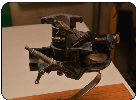
A cut a way display showing the internal operating components of a Zenith carburetor
