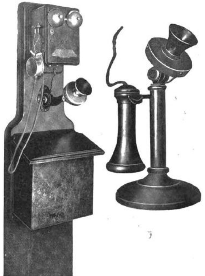
FIG. 7.—DESK SET AND WALL TELEPHONE SET.
