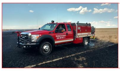
2016 Cascade Fire Equipment Wildland Engine Ford F-550 4X4 400 gallons water 15 gallons foam 125 gallon per minute pump
