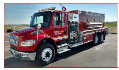
2015 Boise Mobile Equipment Freightliner Water Tender 2500 gallons water 30 gallons foam 500 gallon per minute pump
