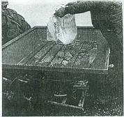
The sieve removes lumps, stones etc. from the fertilizer and thus you avoid incorrect dosing and damage to the spreading unit.
