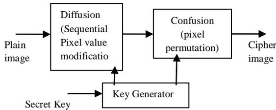
Figure 1. Architecture of Chaos-based image cryptosystem
