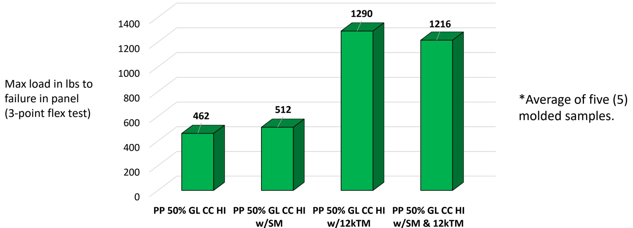
NOTE: Samples molded by inserting spacers on each side to produce fully packed samples
