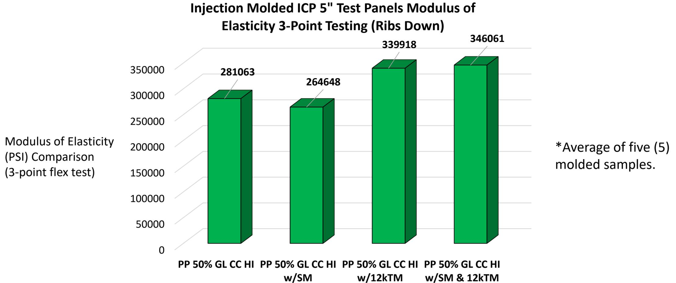
NOTE: Samples molded by inserting spacers on each side to produce fully packed samples
