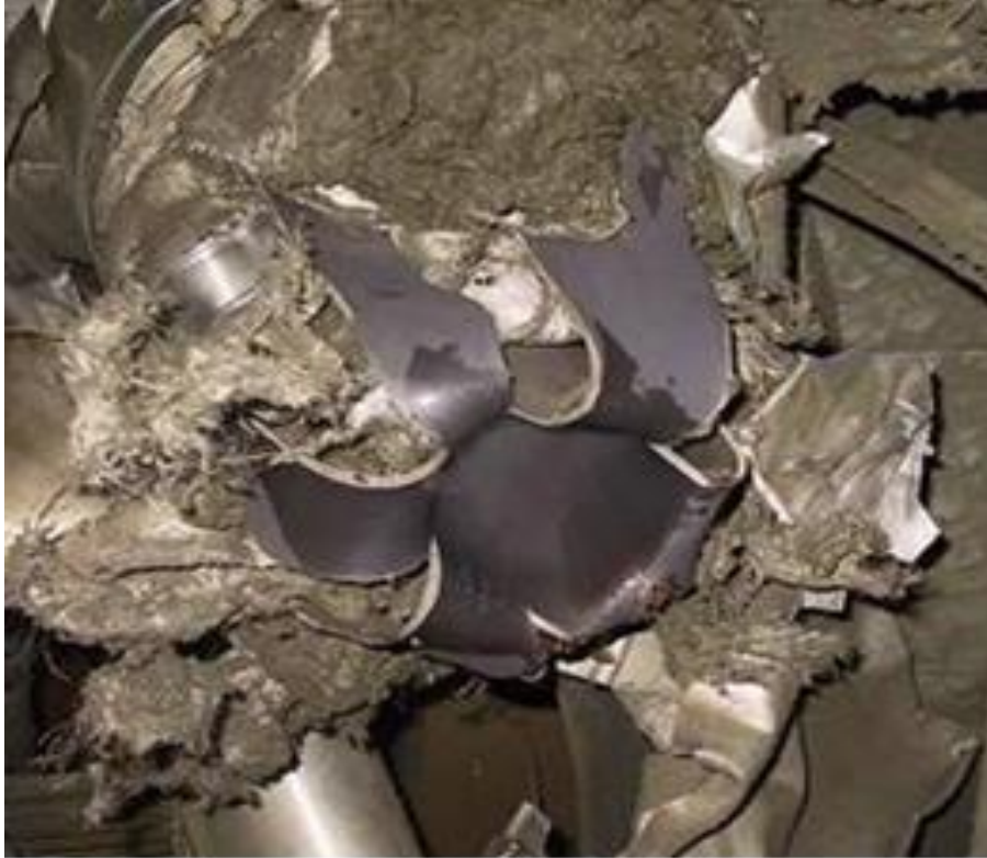
Figure 3: Pump operations and check valve closure in Brunstüttel, Germany autoignited hydrogen and exploded a 6 inch diameter, 1/4 inch thick steel pipe.
