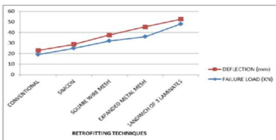
Chart 3 Failure Load & Deflection of all Beams
