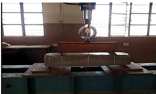
Fig 5.4 Testing of retrofitted beam under Loading Frame
