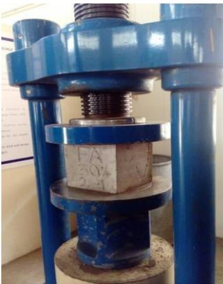
Fig 5.2 Compression testing
