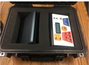
PQsim, BB12hr (underneath), cables, and charger SS1400 12x9x6 (approx)
