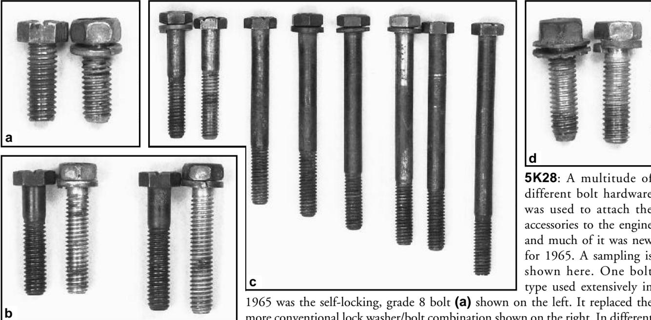
**5K28:** A multitude of different bolt hardware was used to attach the accessories to the engine and much of it was new for 1965. A sampling is shown here. One bolt type used extensively in
