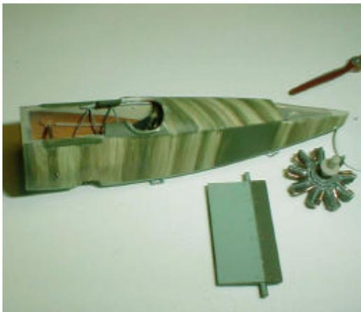
with brown for a wood effect, and the seat black. The sidewall detail was added from 3 triangles of wood grain decal and some gray stretched sprue (for the plywood fairings and steel tube structure). A compass was fabricated from 2 pieces of stretched sprue and a brass bezel from a Tom's Modelworks photo
