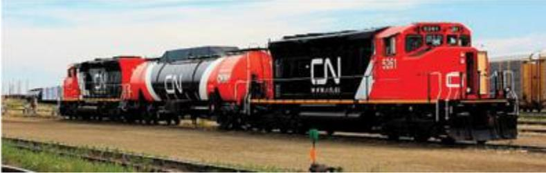
CN's current LNG development program, which began in 2012, uses two EMD 3,000hp SD40-2s equipped with modified 16-645E3 engines. The engines have been converted to LNG using available kits. A 27,000-gallon LNG tender (built in 1992 for UP and on lease from UP) was modified for this program, which Transport Canada approved. The tender was outfitted with a locomotive coolant loop for gasification, filling, and purging arrangements; a power supply; and other equipment.
