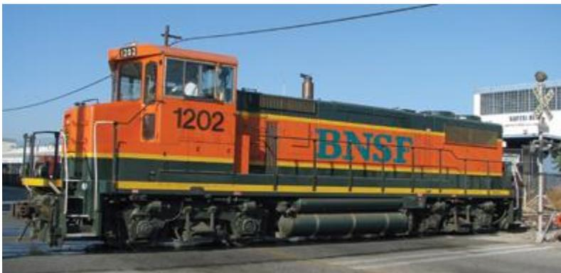
In 1994, Morrison-Knudsen (now the MotivePower Industries division of Wabtec Corp., Boise, Idaho) built four LNG-fueled MK1200G switchers, two each for BN and UP. These 1,200-hp, 100% LNG units were equipped with a 16-cylinder Caterpillar 3516 natural gas spark ignition engine that delivered a 25% to 35% BTU/HP savings over a diesel-fueled GP38-2. All four eventually went to BNSF; they worked in Southern California over the past decade, and were refueled by LNG tank trucks.
