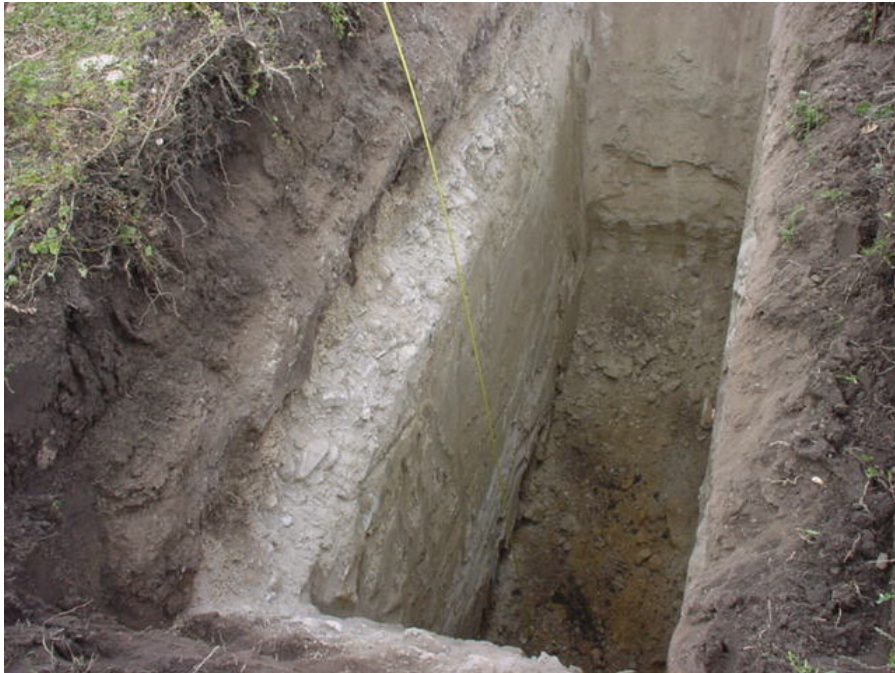
Figure 6: Test Pit 5 soil profile.
