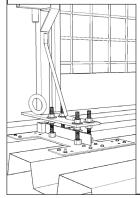
The EMBED steel deck attachment plate is designed specifically for composite slab construction. It is suitable for steel deck 22 GA or thicker, and for the various common deck profiles, including 1½", 2" and 3" composite deck.
