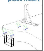
This is an excellent and robust method of attaching to poured concrete slabs. Installation is simple and quick, and the fall arrest tie off anchor can be used as soon as the posts are correctly anchored in place.
