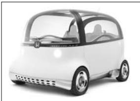
Japan has long been known for odd and whimsical concept cars, and the Honda Puyo is no exception. It's powered by fuel cells, and all four wheels can turn, allowing it to spin 360° in place, but the odd-
