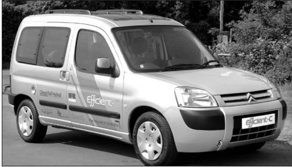
In June 2006 Ricardo, QinetiQ and PSA Peugeot-Citroën unveiled their 100 g/km CO<sub>2</sub> Efficient-C full hybrid diesel demonstrator vehicle based on a Citroën Berlingo Multispace. While the vehicle worked, the project partners estimated that its incremental manufacturing cost needed to be reduced by around 50 per cent (to approximately 2,000) for the technology to become fully commercially viable based on prevailing fuel prices and consumer fiscal incentives.
