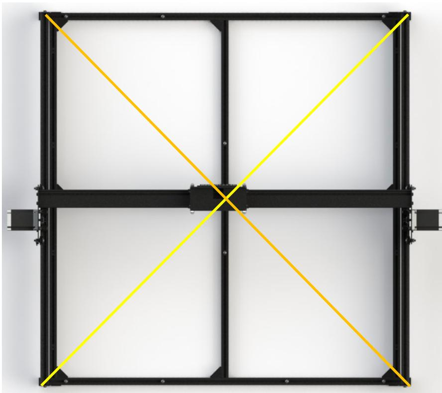
Now cross check the top of the Y rails. The 2 dimensions should be the same or very close.
