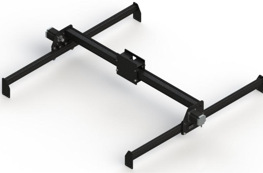
The upper assembly should be together. The best way to do that is allow the rail to relax and be in the same position in the mounting holes. You do that by setting the assembly on a very flat surface like a pool table. Then loosen the 8 screws on the Y end plates to the Y rails. Then tighten them one at a time. There is at least .1mm of slop in those holes and you want all of them in the same position, bottomed out on the hole.
