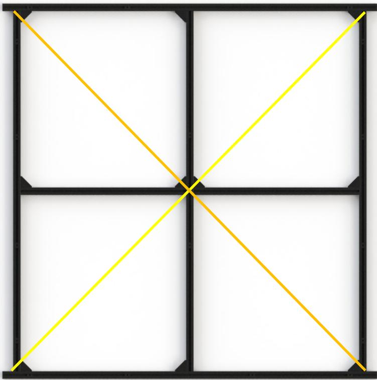
Next cross check the opposite corners of the shorter extrusions, NOT the stick out parts. They should be exactly the same or within 1/32".
