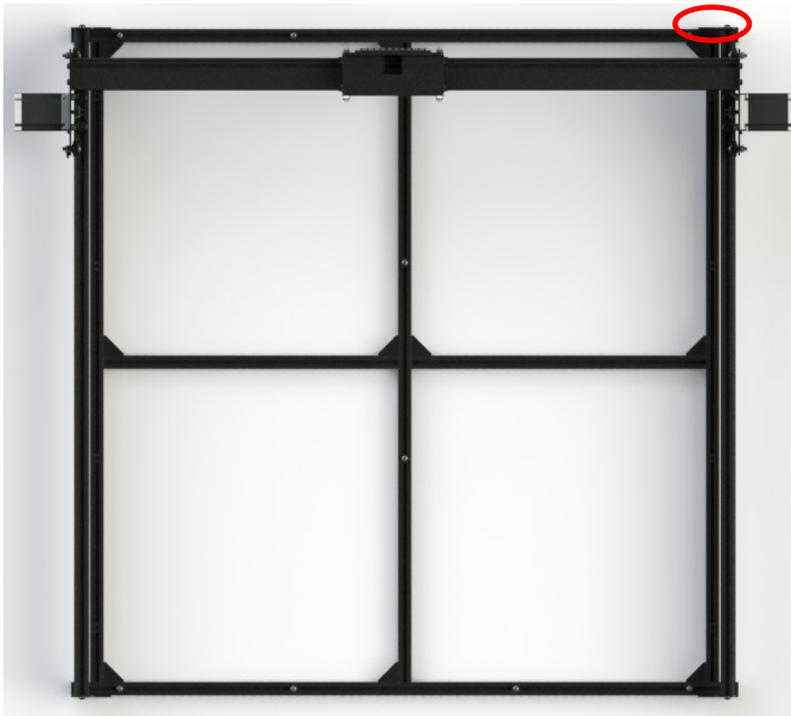
Next slide the gantry all the way to the back. Then tighten the rear Y end plate.
