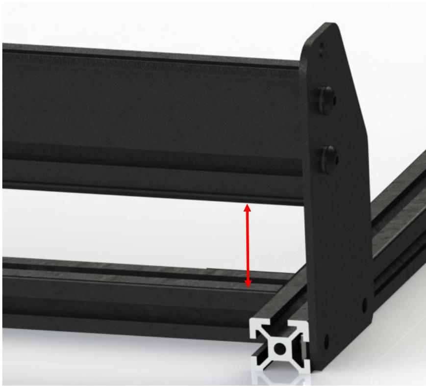
At each of the 4 corners, measure from the top of the base extrusions to the bottom of the Y rails. All 4 should be equal.
