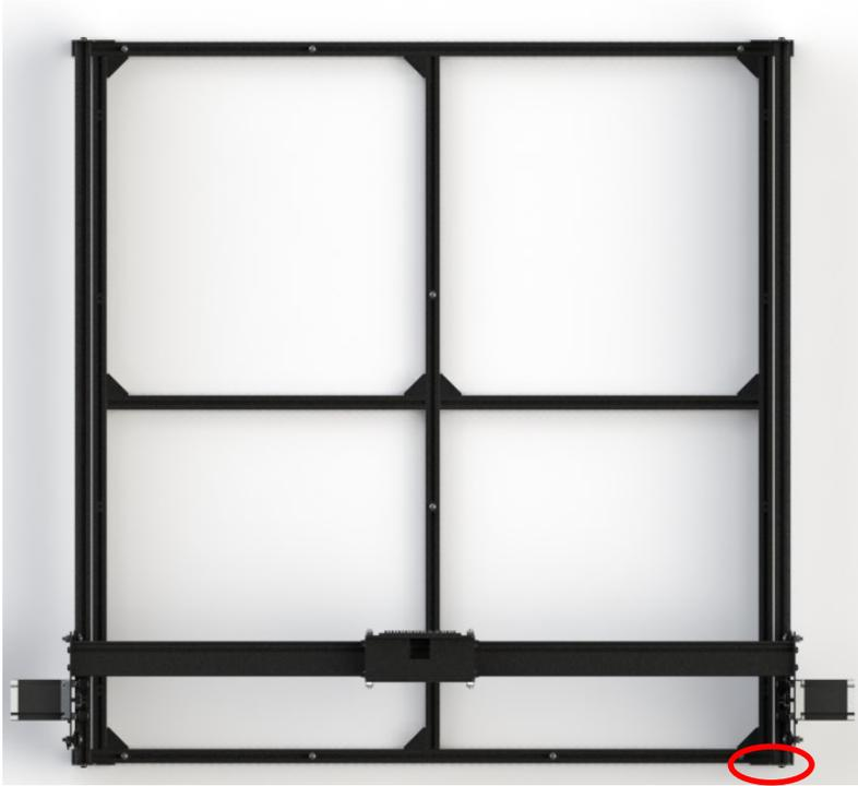
Next slide the gantry all the way to the front. Then tighten the front Y end plate.
