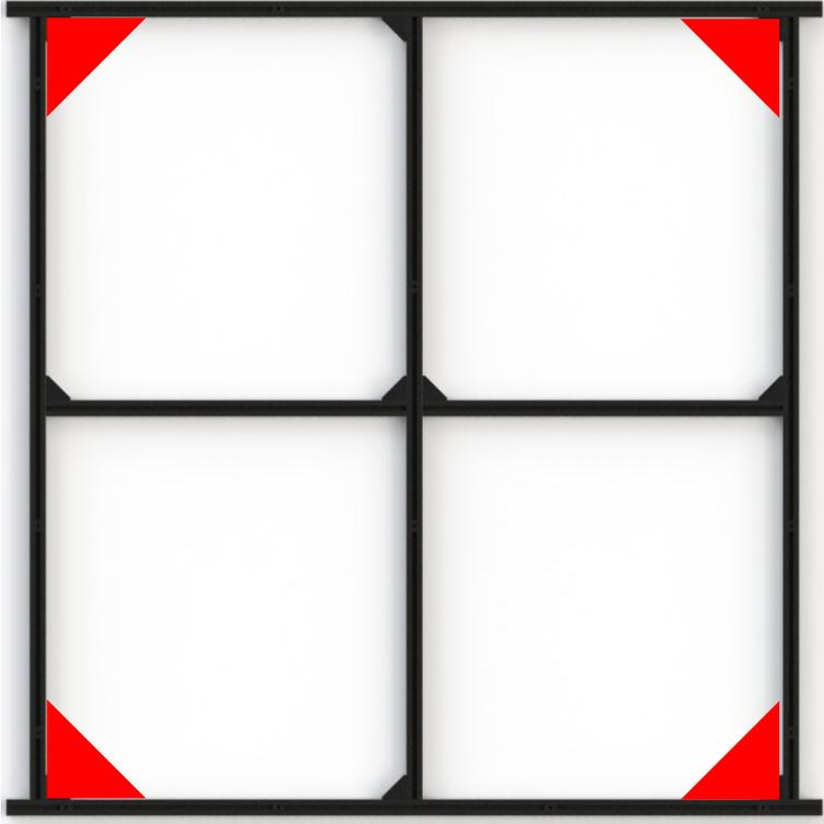
First square the 4 corners. It is more important to be square than it is to have no gaps. The cast corner brackets are very strong and capable of spanning gaps. Try to make the stick out even for the longer extrusions although they don't have to be perfect.
