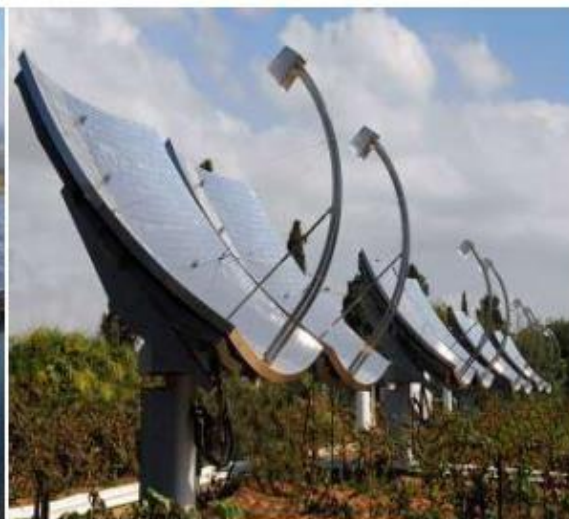
COMBINED HEAT & POWER SOLAR DISH
