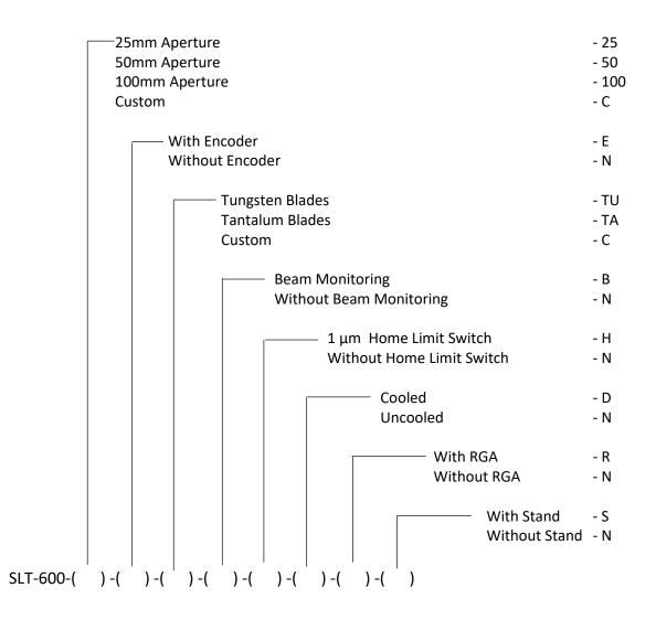
For example, a chamber configured with 25mm Apperture, with an Encoder, Tungsten Blades, 1  $\mu$ m Home Limit Switch, Uncooled, without RGA and a Stand would be denoted by: SLT-600-25-E-T-H-U-N-S
