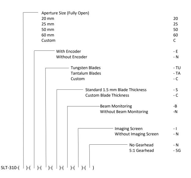
For example, a chamber configured for 25mm Aperture, No Encoder, Tungsten Blades, Standard Thickness, Beam Monitoring, Without Imaging Screen, with no gearhead would be denoted by: SLT-310-25-N-TU-S-B-N-N.
