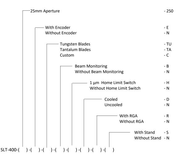
For example, a chamber configured with 25mm Apperture, with an Encoder, Tungsten Blades, without beam monitoring, 1  $\mu$ m Home Limit Switch, Cooled, without RGA and a Stand would be denoted by:
