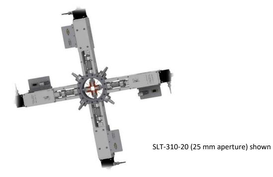
The SLT-310 series slits are designed for UHV and can be used for apertures up to 60 mm. Blades are actuated independently by 4 actuators mounted on the slit body. This slit system is designed to be mounted inside a variety of different ConFlat flanges.
