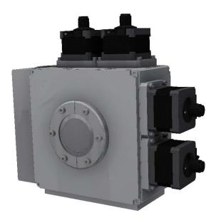
These high-precision slits systems consist of four blades that are housed in an aluminum body. These slits use standard micro-stepped stepper motors that can be controlled with a wide array of controllers/drivers available on the market. The design incorporates mechanical limit switches.
