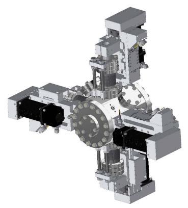
The SLT 400-250 slit system is designed for UHV and can be used for apertures up to 25 mm x 25 mm. Blades are actuated independently by 4 actuators mounted on the slit body. This slit system was designed to be robust and easily serviceable.
