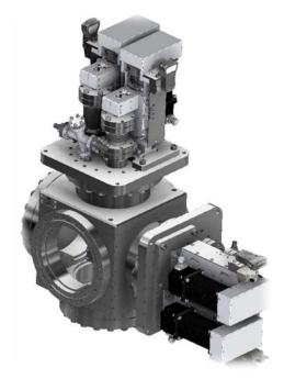
The SLT-600 slit system is designed for UHV and can be used for apertures from 25 mm x 25 mm all the way up to 100 mm x 100 mm. Blades are actuated independently by 4 actuators mounted on the slit body. This slit system was designed to be robust and easily serviceable. AVS|US draws from an array of standard components to rapidly develop a reliable solution to each beamline's needs.
