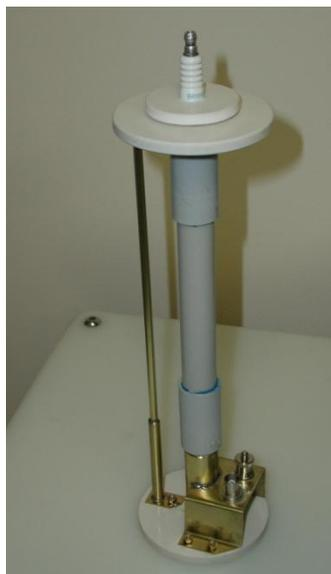
Therefore, the technical problem becomes how to accurately scale down a typical 30kV voltage to the input of a recording device such as an oscilloscope which has a 1 Meg Ohm and 15pF input impedance while still maintaining a broad frequency response so that the recorded wave maintains its original shape and so the oscilloscope itself is not at risk of damage.
