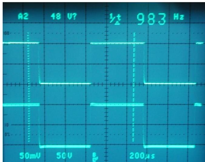
The upper trace is the input voltage which is a near 1kHz 100v peak to peak square wave from the PG506 generator. The lower trace is the output voltage which is close to 100mV pp. The Cal resistor was then added to gain the exact DC step-down ratio. (Without the compensation capacitor network consisting of the brass rod and 1300pF capacitor,
