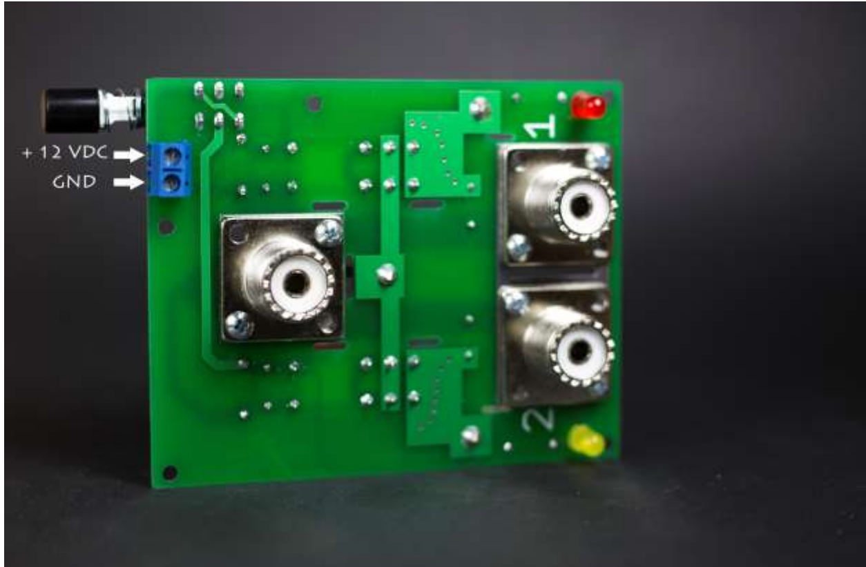
Photo 2 - Power connection detail - Make sure to observe correct polarity
