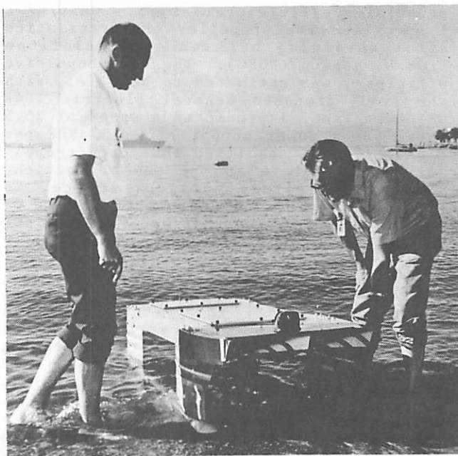
Figure 4. Five-foot, 6-channel, radio-controlled model of the KAIMALINO being prepared for tests in San Diego Bay by D.T. Higdon (left) and C.R. Nisewanger (right). (U.S. Navy photograph)
