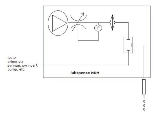
\* External priming source, syringe pump, peristaltic pump, manual syringe etc required to prime and fill dispense module. Can be primed either forward flow (dispense) from bulk reagent reservoir or reverse flow (aspirated) from source reservoir, microtiter plate etc.
