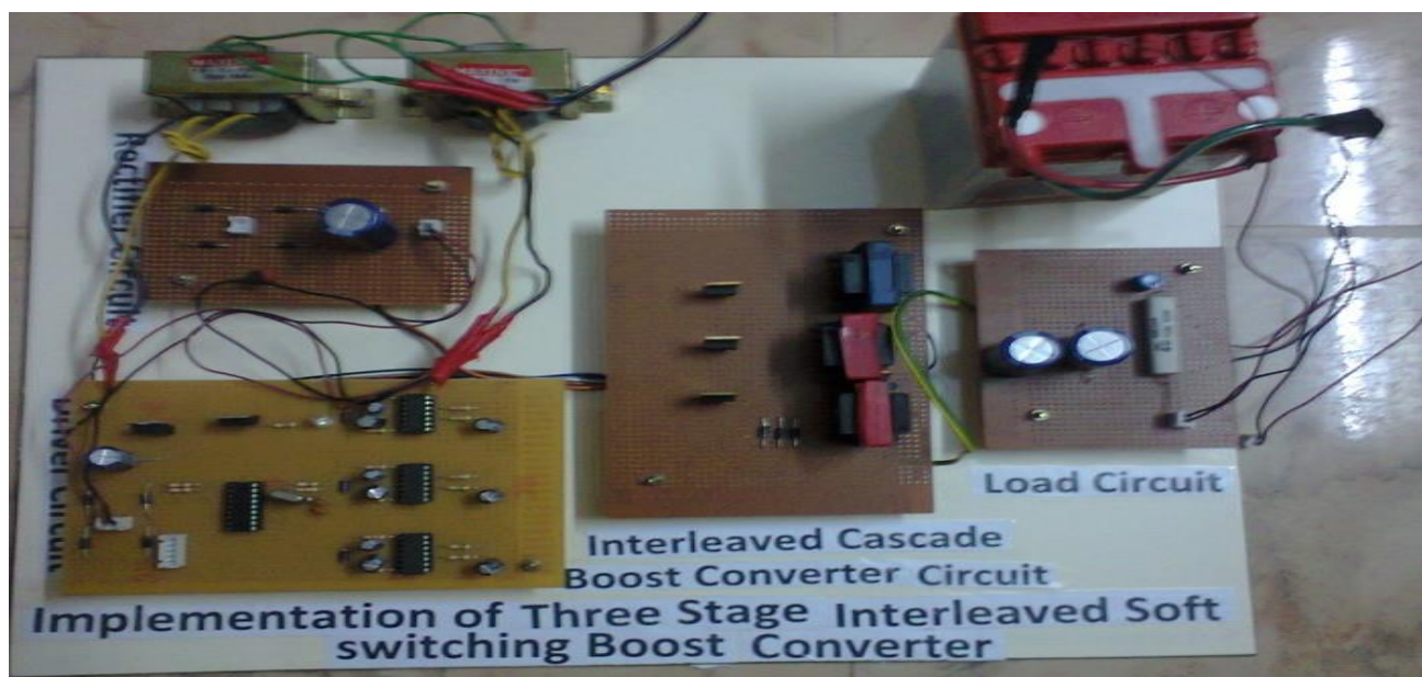
Fig. 9. Experiment result of interleaved soft switching boost converter
