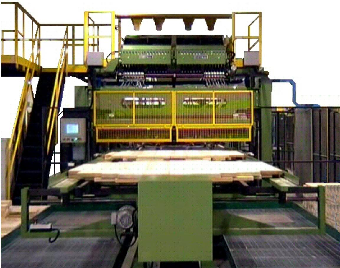
Automatic nailing machine with 32 nails to assemble cable drum flanges, consisting of:
