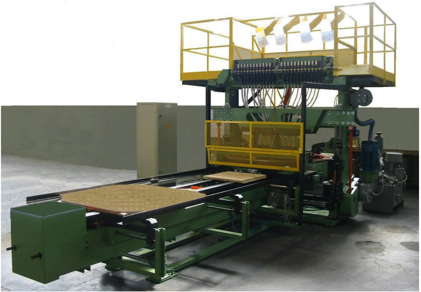
Automatic nailing machine with 22 nails to assemble cable drum flanges, consisting of:
