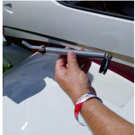
Dave Jalanti is showing a potential customer his newly developed pitch trim spring. Dave sells this Lightning mod that helps to trim off the nose-down pitch feel when the flaps are down and your aircraft is at a light weight.
