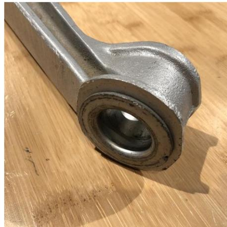
***Control Arm Prepared for Bushing Installation***
