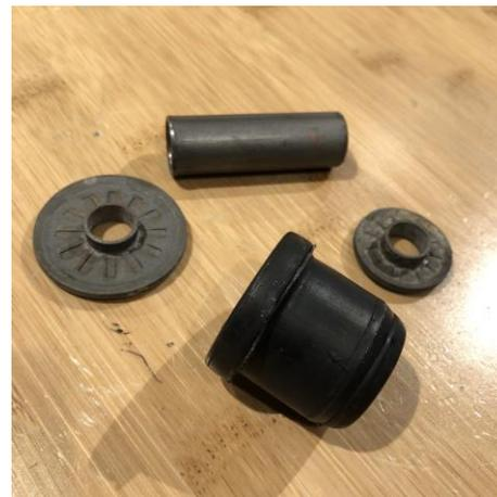
***Components of the OEM Rubber Bushing***
