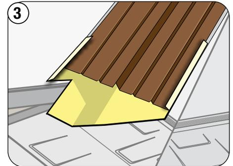
**3** Fit Valley metal over and onto the formed exit tray and embed the Valley into the sealant.
