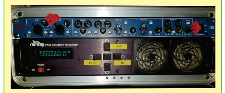
transmitter works on the regular FM broadcast band, the same that you listen to in your car or home. Not a toy, this is capable of transmitter power up to 50 watts (for use out of the US of course) on a frequency selected by you. It is capable of stereo or mono operation. It is contained in a 3 space rack case and powered by 110 VAC. It has provision to connect a 12 volt battery to it that takes over powering the transmitter automatically in case the AC power fails.
