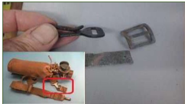
Clip and buckle from the 'walk around' oxygen cylinder that secured it to the table. This also allowed the crew member to walk freely at a great height. (Coll. J. Hendrix)
