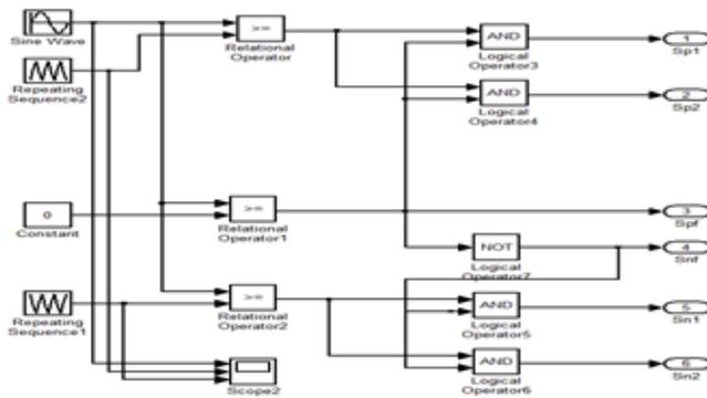
Fig11: block diagram with four HF legs
