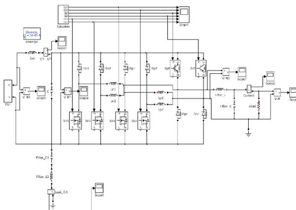
Fig18: two leg circuit diagram for existing system
