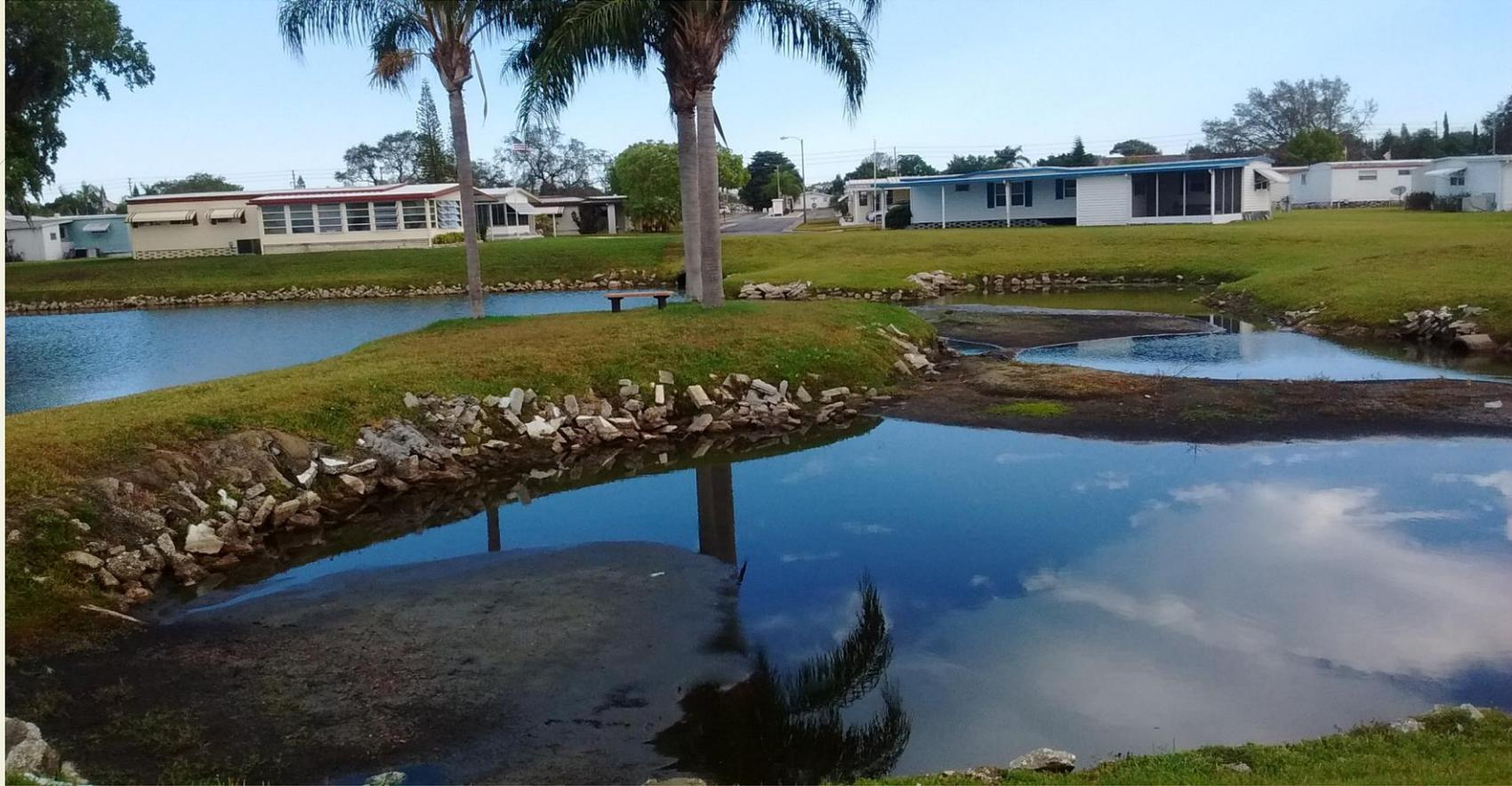
Silt build up in this pond adds to continued flooding on Moog Road and Jarvis Street. Pond to be dredged in order to allow proper water flow.
