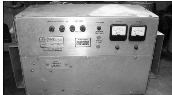
Lester Electrical 12/96 volt Battery Charger, 208/230 volt input, 96 volt 30 amp output, used by Jet Industries in converted trucks. \$50.00
