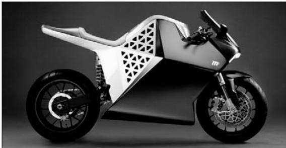
— not bad for their first time at the event. There's a nice record of all that occurred at <http://ridemission.com/blog>. Some technical specs include a lithium-ion battery pack with thermal management, a liquid-cooled, 3-phase AC induction motor rated for 100 lb-ft of torque at 0 to 6500 rpm and range of 150 miles per charge.
