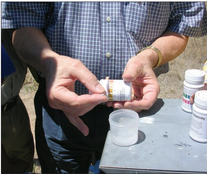
Field test to identify the pH and alkalinity to allow for proper buffering of the chlorine solution for effective disinfection.
