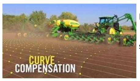
Maintains accurate seed population and spacing on curves by slowing down the inner row units and speeding up the outer row units on curves
