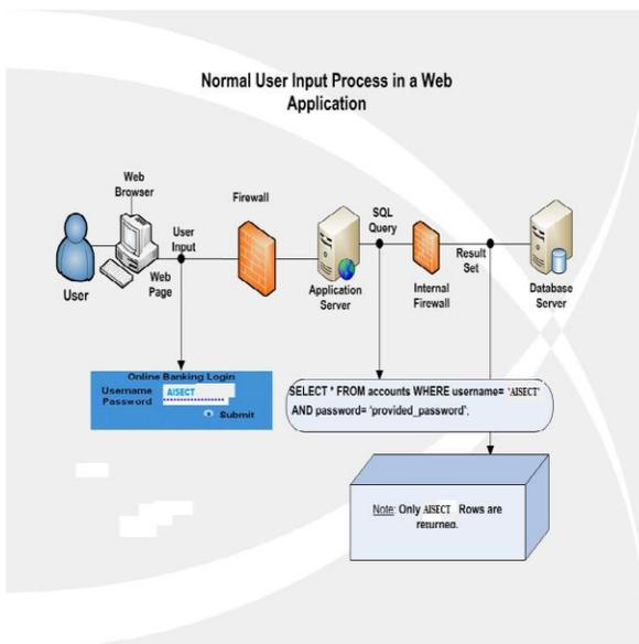
Fig. 1: Architecture of user input process of a Web application
